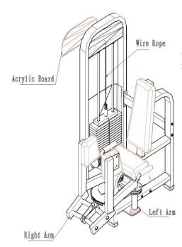
Install the left and right arm, and string the wire rope, and install the acrylic board finally.
